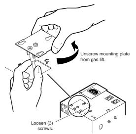
Figure 3-5 — Removing the gas lift mounting plate
